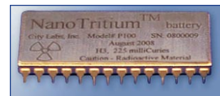
La pila NanoTritium (© City Labs).
