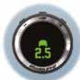
The system gauges the distance to the vehicle ahead and warns if the headway is insufficient.
