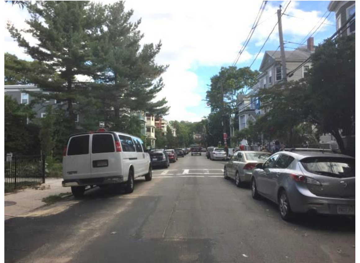
Crosswalk without daylighting
