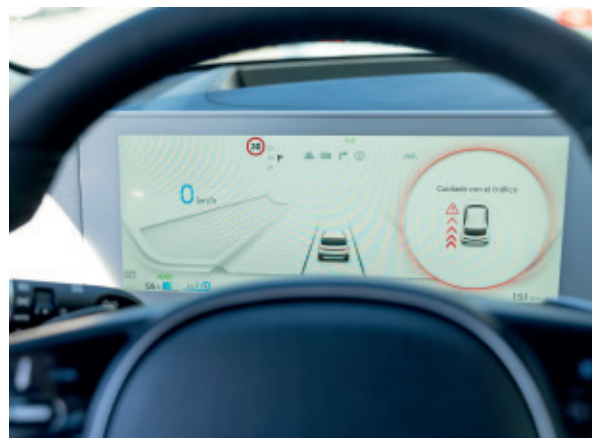
Exit Warning System
