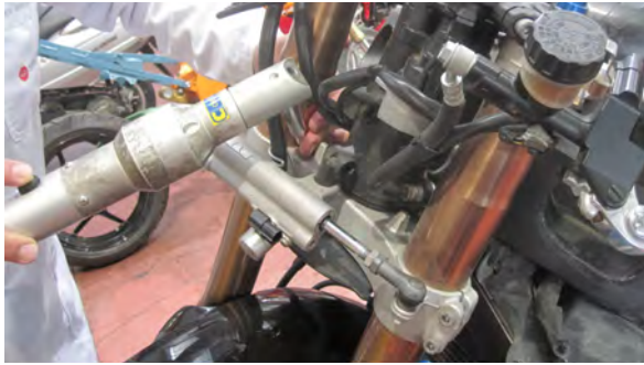
Control dimensional de tija inferior
