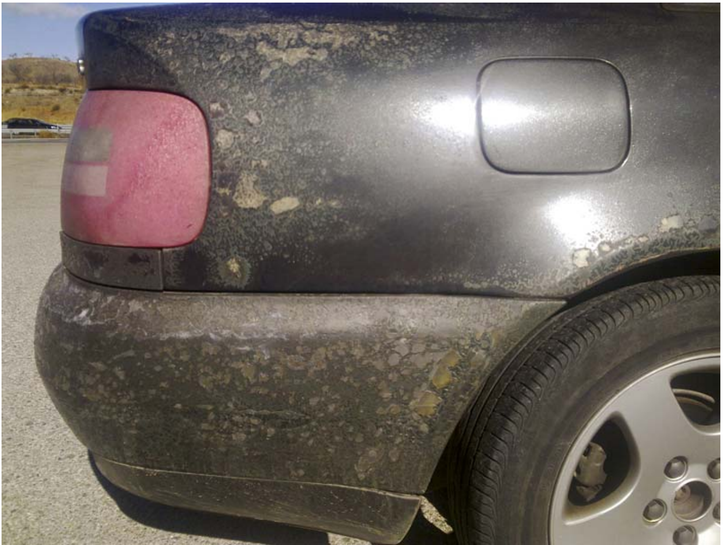
Figure 11. Radiation marks on a nearby vehicle. Source (4) ; Authors
