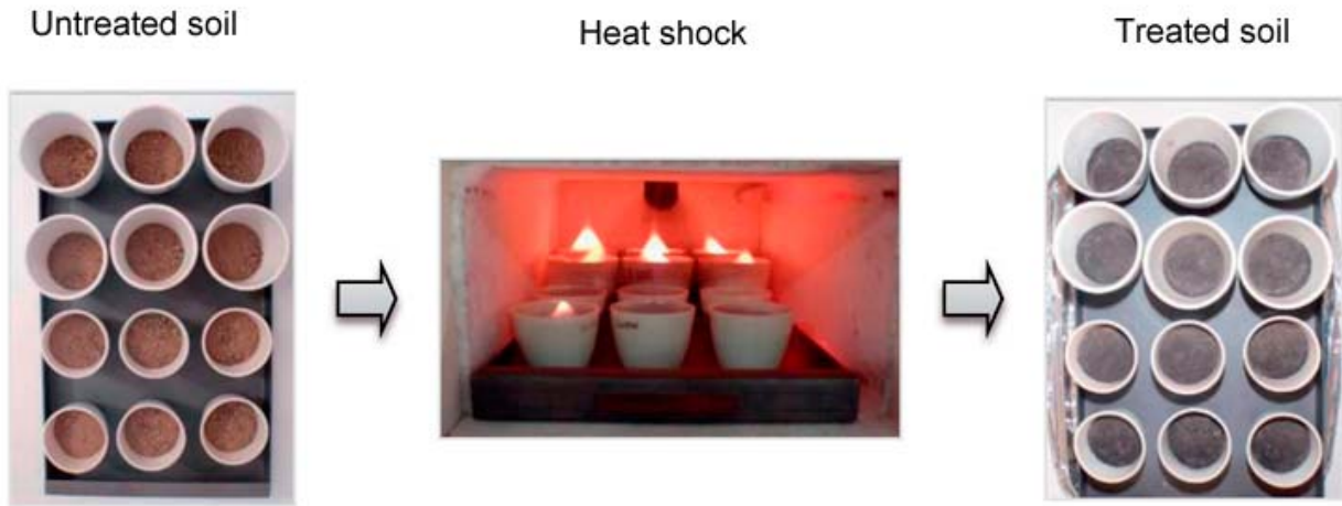
Figure 2. Treatment of the soil samples: heavy-soil sampling aliquots ready for treatment; heat shock treatment in muffle furnace and post-treatment appearance of the samples
