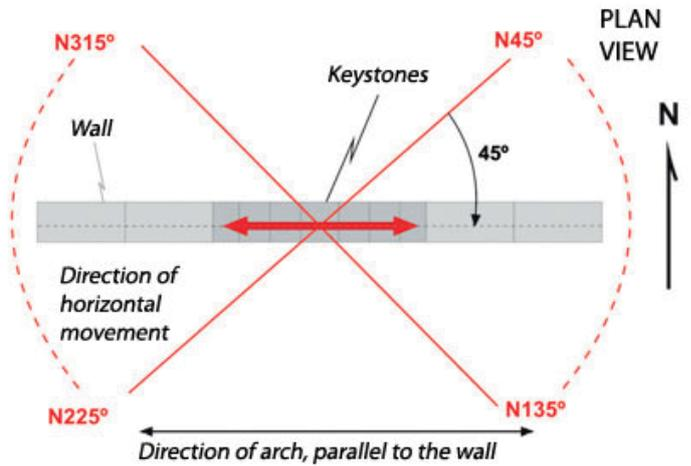
Figure 5. Idealised schemes of deformation analysis in arches and lintels. a) Deformation of seismic origin that shifted the keystones horizontally; the direction of maximum horizontal shortening ( $e_y$ ) is analysed in a similar way to that of titled walls. b) Deformation of seismic origin causing dropped keystones; the direction of  $e_y$  lies at an angle of less than  $45^\circ$  vis-à-vis the plane of the arch-containing wall.
