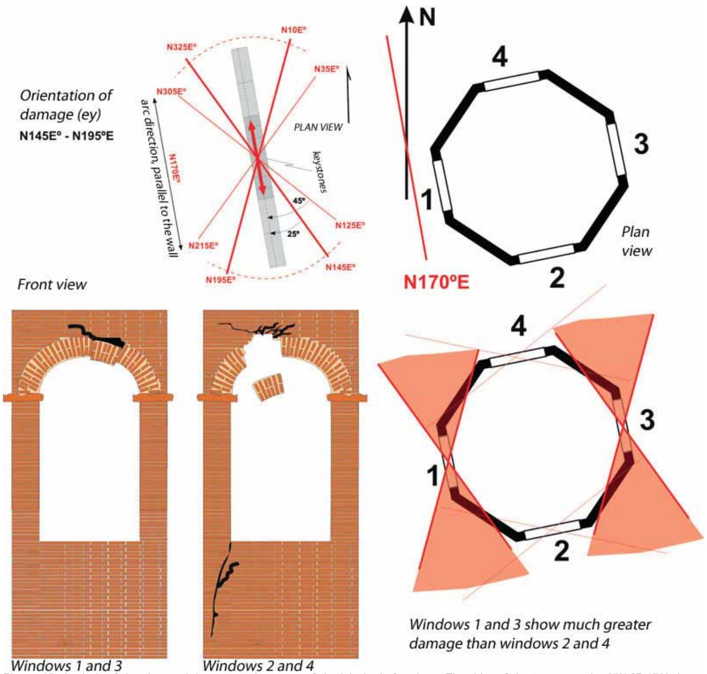
Figure 15. Analysis of the observed damage to the tower of the iglesia de San Juan. The sides of the tower running NW-SE 170° show more damage than those running in other directions. Determination of these orientations enables us to quantify the earthquake-caused deformation.
