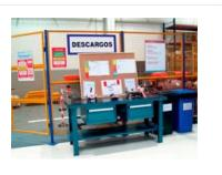
Station designed to steep participants in clearance and tagout procedures. Stress is laid on the various tagging systems and hold cards used during the clearance processes.
