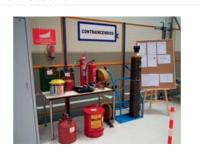
Drills here involve the proper management of flammable material in due accordance with plant procedures (labelling, storage in airtight cabinets, etc). The station includes related signage and recreates measures for reducing the fire load in cubicles.
