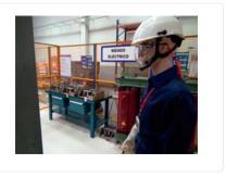
A cubicle recreates a motor control centre with electrical switches of varying power to simulate situations faced by operators of electrical equipment.
