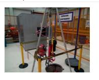
This has two separate spaces simulating a tank and a gallery or sewer. Practical working activities are carried out in them, rehearsing the steps to be followed in confined-space working and rescue techniques. Temperature conditions can be modified in this station (heat stress).
