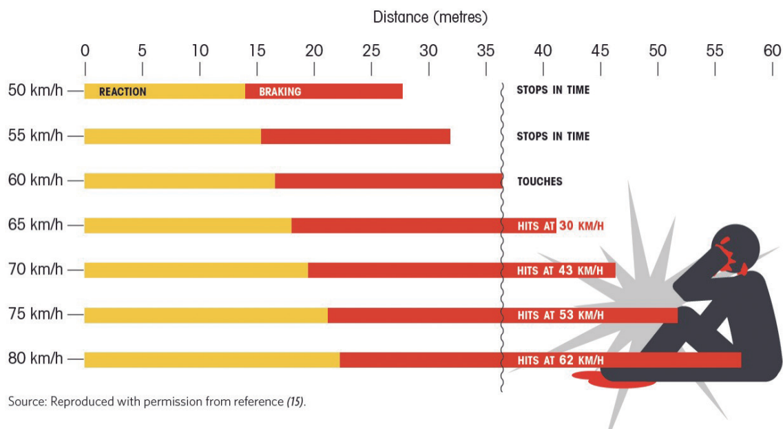
FIGURE 17. STOPPING DISTANCE AT DIFFERENT SPEEDS (ALLOWING A REACTION TIME OF APPROXIMATELY 1 SECOND)
