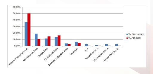
Nevertheless, despite attempts to analyze the cause of breakdowns, very often the reason for the failure is not known due to the difficulties in reconstructing the damage and research with the manufacturer who is the guarantor of the correct design of the equipment.
