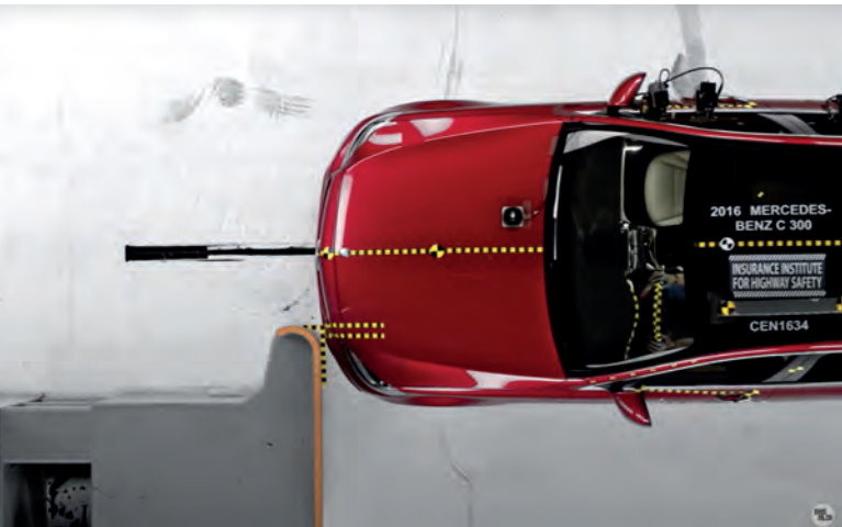
Ensayo small overlap realizado por IIHS
